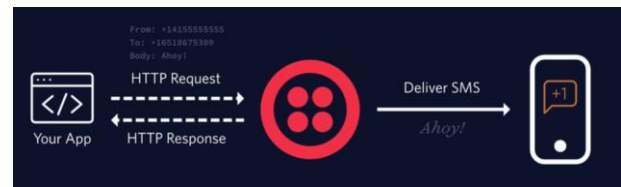
Figure 3: Architectural diagram of Twilio integration In the above diagram says that, website sends the HTTP request to Twilio and Twilio send back the response to that request and simultaneously it sends SMS and call to phone which defined as emergency contact.
