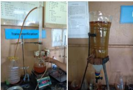
Figure 3: Trans-esterification Setup & Settling Vessel
