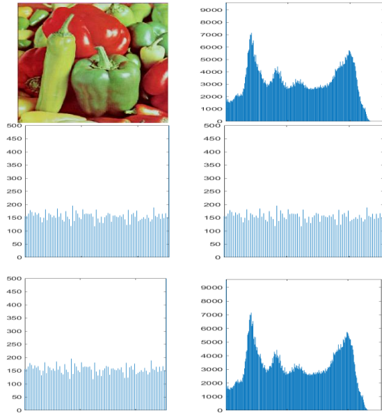
Figure 5: Original input image, Histograms of input, ciphers of scrambled (R-, G- & B-channels) & descrambled images.
