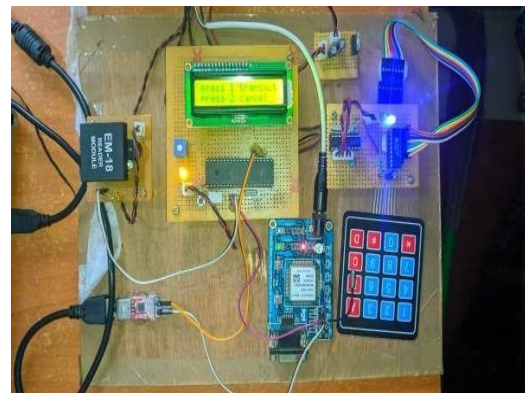
Figure 7: Hardware connection circuit of proposed face authentication system
