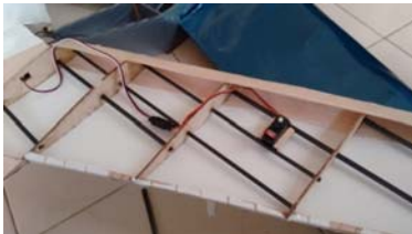
Figure4.6 Servo fixture on the top wing to control the elevon.elevon.
