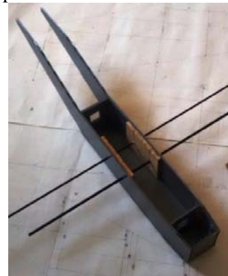
Figure 4.1: Fuselage fabrication using hollow polycarbonate sheet.
