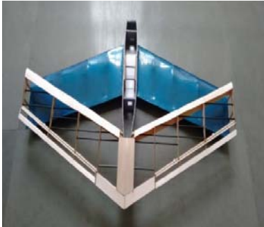
Figure4.5Elevons fabricated for the top wing
