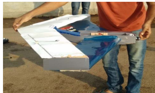
Figure 4.11: Verification of position of CG Along Z axis.
