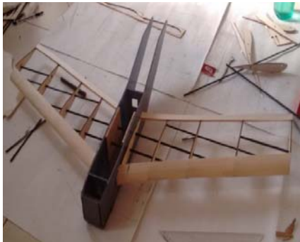
Figure 4.2: Leading edge and trailing edge of the bottom wing
