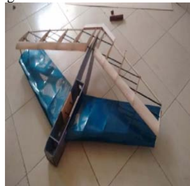
Figure 4.4: Skeleton of the top wing before fixing elevon.
