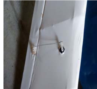
Figure 4.7: Connecting rod fixed between the servo arm and the control hon.
