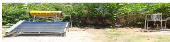
Fig1: Schematic diagram of Solar Assisted prototype biodiesel production plant
