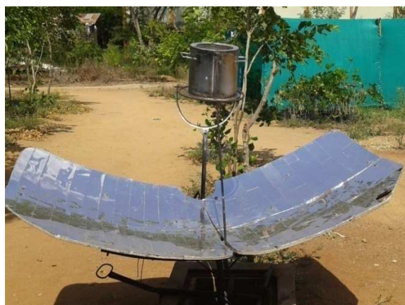
Plate 1. Rice cooking using Butterfly type Solar Collector
