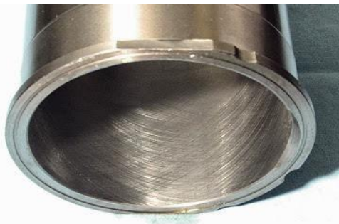
Figure:2 Cross hatch pattern on a cylinder
